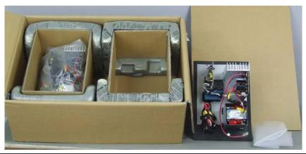
NOTES: Parts must be in a plastic bag and securely packaged to prevent damage. Apply labels to inner and master carton with KRK part number, description, shipping weight, and shipping dimensions.
