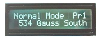
In normal mode the meter shows continuously gauss value and polarity....
