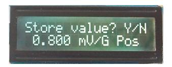
If you use the small pcb for probe with A1302 and AD22151 and respect the right wiring\*\* between probe and main unit you will have sensor A1302 as PR1 and you have to enter 1.300 mV/Gauss for it in calibration menu. You will have then sensor AD22151 as PR2 and you have to enter 0.400 mV/Gauss for it in calibration menu.
