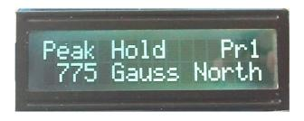
In peak hold mode meter takes measure continuously but shows highest value measured... it resets when value returns to zero or when magnet polarity changes...
