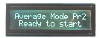
in average mode, meter takes 131070 measures and shows average value.... it could be useful to know average gauss value in a bar magnet (moving probe along magnet while measuring)...
