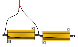
Two 120 ohm resistors wired in parallel for equivalent 60 ohms replacement of original value resistor. To run power tubes cooler, use higher value aluminum resistors such as 150 ohm for equivalent 75 ohms. This will further reduce heat in the chassis
