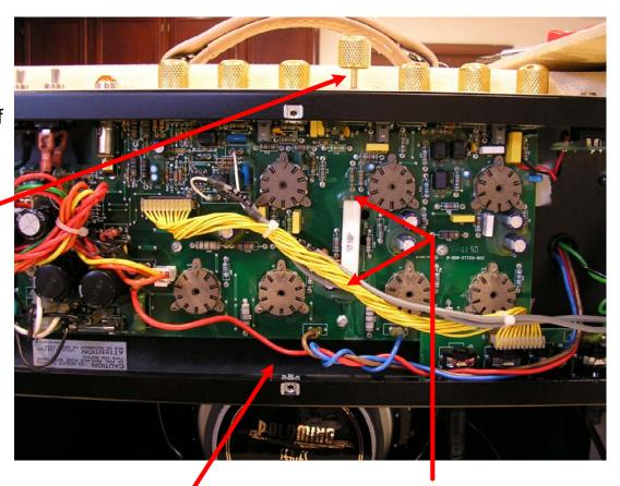
Mount two resistors on bottom of chassis here.
