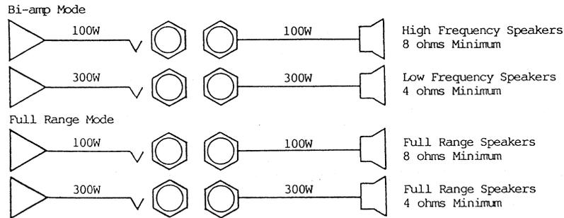
**CAUTION:** Under no circumstances should the 100W and 300W outputs be connected together or to the same speaker!
