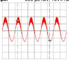
Input Signal:  $\sin$ ; 1 kHz; 0,7V<sub>RMS</sub> Scope:  $500 \mu s /div$ ; 20V = /div
