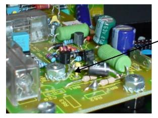
mounted with soldering lug
