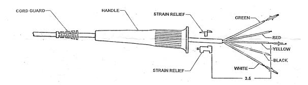
Weller EC232 EC1201A and EC1201P Handle and Cord Guard
