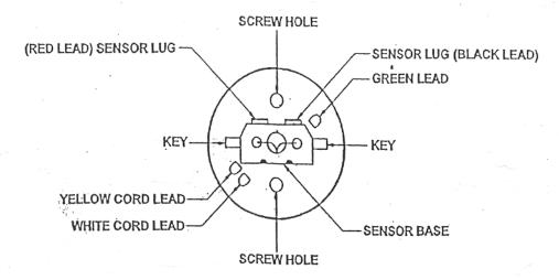
View of black heat insulator from handle/cord side EC1201P or EC1201A
