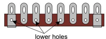
12) Connect the remaining 470K resistor to terminal #10 and insert the other end through the lower hole of terminal #12. **Now, solder** the lower hole connections at terminal #12.
