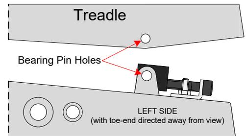
*Tip: Lay the pedal on its side with a couple of magazines stacked underneath the treadle, on the side opposite from where you will be hammering, to keep the treadle propped up from your work bench.*
