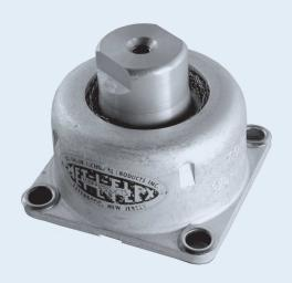
The high damping and nonlinear characteristics of MET-L-FLEX load carrying element and limiter pads in the all metal 1201 and 1202 Series Isolators assure controlled shock and vibration isolation protection for mounted equipment.
