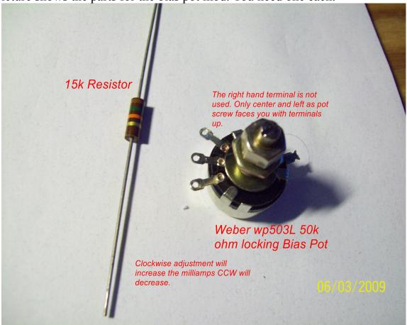
To start, I inserted my bias probes and took readings on each tube before proceeding and recorded those readings. I also took readings across the 15k resistor touched at left terminal and probed center terminal. I then preset the resistance for pot with 15k resistor to 33k. Same as the resistor you will be removing. Using alligator leads on the terminals and your multimeter leads so you can adjust setting.
