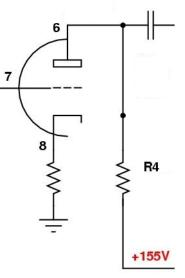
**Ex. 1c)** If the power amp stage cathode resistor R10 measures 150 ohms and the voltage drop across that resistor measures 8.25V, how much current is the tube pulling?
