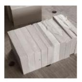
Pieces on the right side, with ragged edges, clearly show wood failure. As you move to the left, you'll notice the smooth edges, which indicate glue failure.
