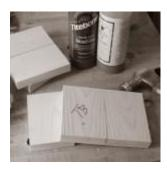
A simple test to determine if joint failure is a result of glue failure or wood failure, is to assemble a few joints then whack the assembly with a hammer. Something has to give. Just hope it's the wood – because that means the glue is stronger than the wood.
