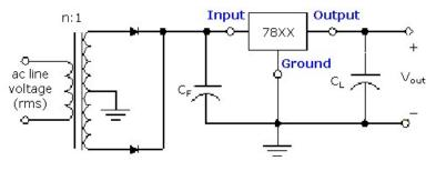
order to design a regulator using one of these ICs, and ensure that the required minimum and maximum input voltages are maintained, we need to select an appropriate transformer and filter capacitor.
