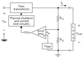
A reference voltage, V<sub>REF</sub>, is compared with the voltage divided output, v<sub>out</sub>. The resulting error voltage, v<sub>e</sub> is given by
