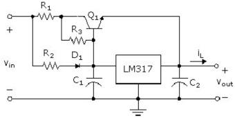
right, allows the output current to increase to about 5A while still preserving the thermal shutdown and short circuit protection of the IC.
