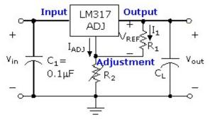
denoted  $R_1$  and  $R_2$  in the figure. As for the 7800 family, the capacitor  $C_L$  is optional. When it is included, the transient response is improved through the rejection of transients that may appear on the regulated supply line. Your author further states that the capacitor  $C_1$  is needed if the device is physically located far from filter capacitors. However, an input bypass capacitor is usually used to short out any high frequency variations that may occur in adjoining circuitry.
