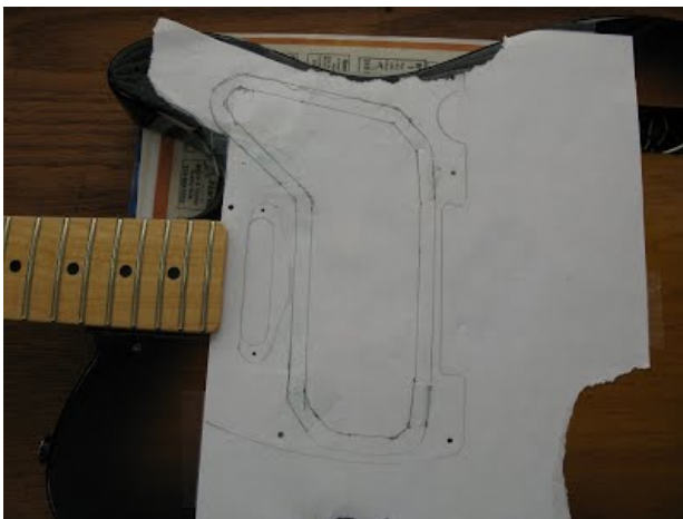
A paper sketch of the pickguard shape and coil groove shape taped to the guitar to guide me in routing
