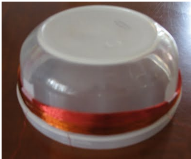
Both coils were wound on a plastic container with 20" circumference
