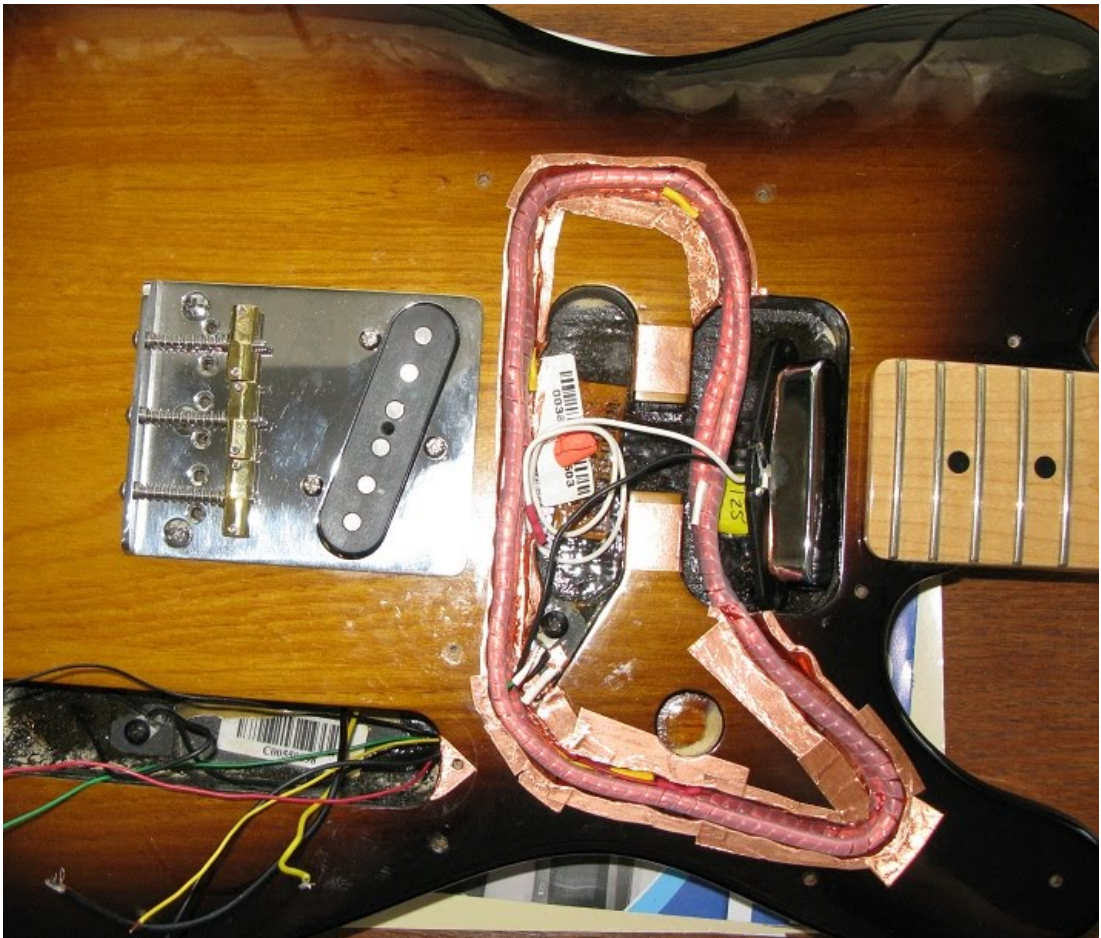
The PUs and coils are put in place for final tuning of the coil taps for the final coil shape Wires from the coils and the PUs are visible extending into the control cavity
