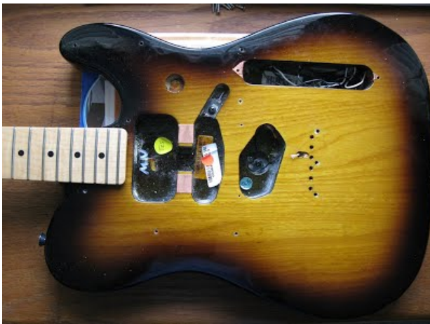
The stripped telecaster before the coil slot is cut with a router
