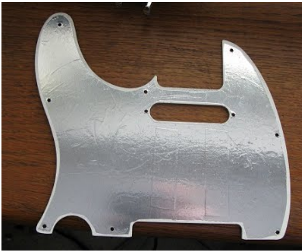
The backside of the pickguard is also shielded. I used spray adhesive and aluminum foil.
