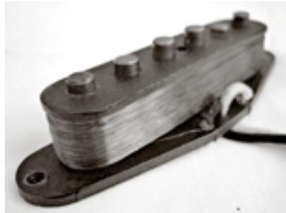
The coil is a big contributor to a pickup's output and tone. The coil wire – the coated copper electrical wire we use to wind a pickup is very fine, generally
