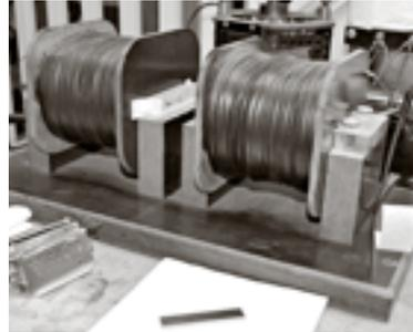
I get Alnico magnets not magnetized and magnetize them myself. I built the magnetizer and beside it is a setup to demagnetize the magnets. There was a time when it was thought that one of
