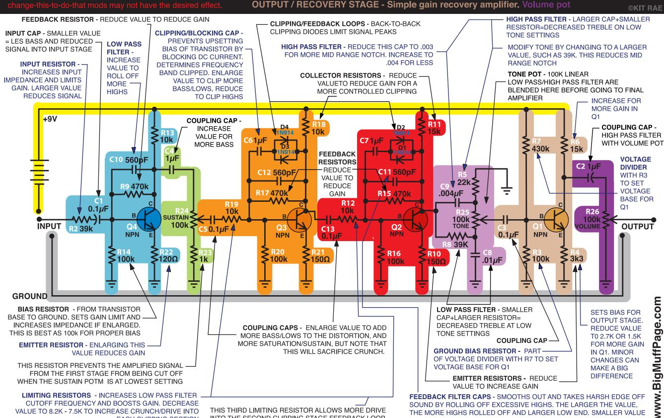
INTO THE SECOND CLIPPING STAGE FEEDBACK LOOP
