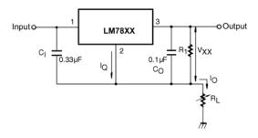
$$I_{O} = \frac{v_{XX}}{R_{1}} + I_{Q}$$
