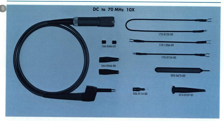
The P6055 is a miniature low-capacitance, 10X Probe designed for use with Tektronix differential amplifiers having nominal input capacitances from 20 pF to 47 pF. The attenuation ratio is adjustable to 10X to compensate for differences in input resistance of the amplifier (the amplifier input resistance must be 1 M $\Omega$   $\pm$  2%). A special locking type readout connector allows the probe to be used with instruments with or without readout capability.
