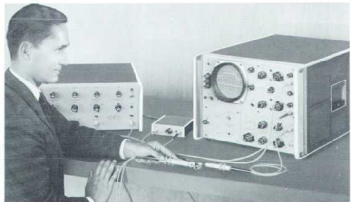
Fig. 3. Typical test setup using new clip-on current probe together with voltage probe to simultaneously observe and measure current and voltage in test circuit.
