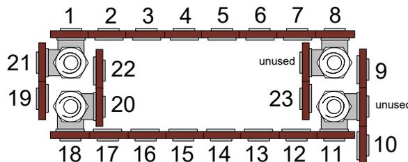
Strip and tin a 6" piece of wire and connect to terminal #19 and the anode (+) terminal on the LED. Solder the connection on the LED and trim the excess lead.
