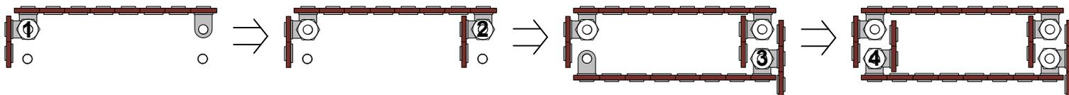
*It may be necessary to angle the terminal strips forward with your fingers so that the terminals are not pressing against the sides of the enclosure making it difficult to mount the components.*
