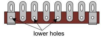
Strip and tin a 5" piece of wire and connect to the input jack's tip lug and terminal #10. *Route this wire along the surface of the enclosure to leave more room when mounting the terminal strip components.*
