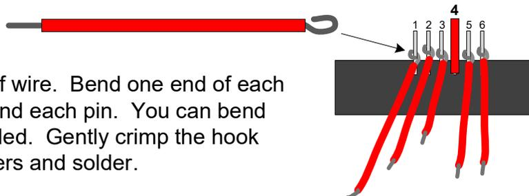
*Be careful not to accidentally short adjacent pins by soldering two wire hook ends too close to each other. You may find it necessary to stagger each hooks placement on the pins.*
