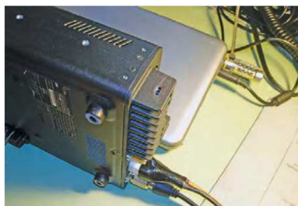
Figure 5 — A small slot cut in the heatsink or metal frame of your radio is all that is needed to accommodate a Kensington lock. [Bob Klaus, NØYWB, photo]
