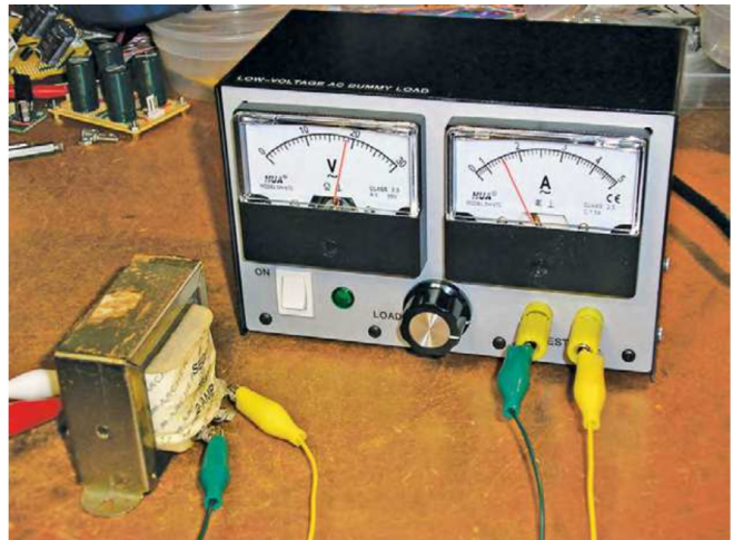
Figure 3 — Testing a transformer with the load. [Bryant Julstrom, KCØZNG, photo]
