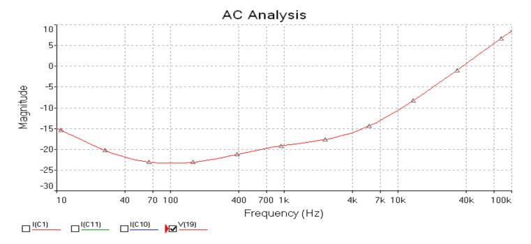
LF boost curve appears to be set by C2 and C10 bootstrap connections from emitter circuits of Q1 & Q2, coupled to the bases by the voltage dividers R2 & R3 for Q1 and R13 & R14 for Q2. HF boost curve set by C4 across the two emitter resistors R6 and R7 to ground. That compensates for the HF rolloff response of the Mic Input Transformer's freq response.
