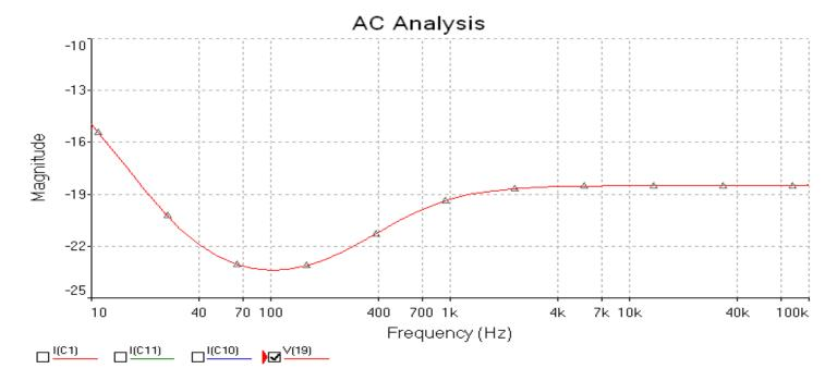
HF boost curve set by C4 across the two emitter resistors R6 and R7 to ground was disconnected for this response curve. LF boost curve appears to be set by C2 and C10 bootstrap connections from emitter circuits of Q1 & Q2, coupled to the bases by the voltage dividers R2 & R3 for Q1 and R13 & R14 for Q2. It looks larger, but that's from reducing the graph range from 30dB to 15dB. Response is relative to the nominal gain of the preamp.
