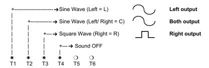
Pressing the buttons as indicated in the following table, you hear the corresponding sounds. Put the volume potentiometer at max.
