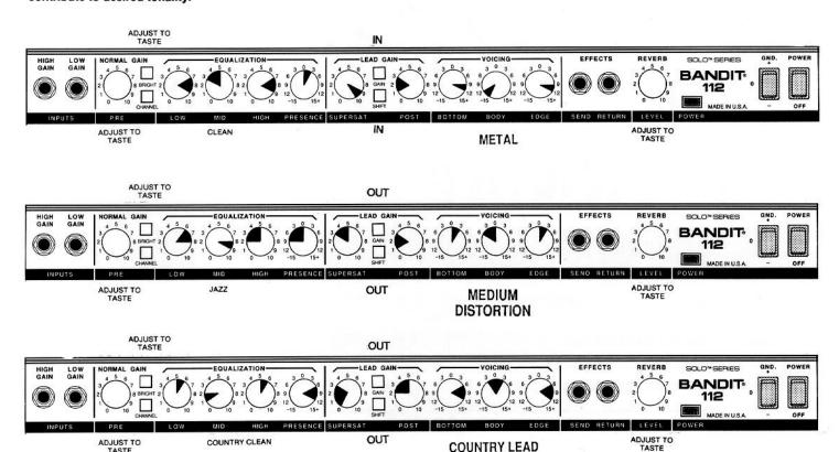
**BANDIT® 112 SPECIFICATIONS RATED POWER & LOAD** 80W RMS into 8 ohms
