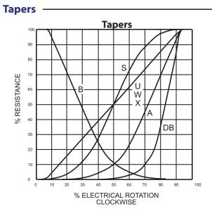
Tapers A, DB, S and U are measured between the wiper and the counter-clockwise terminals;
