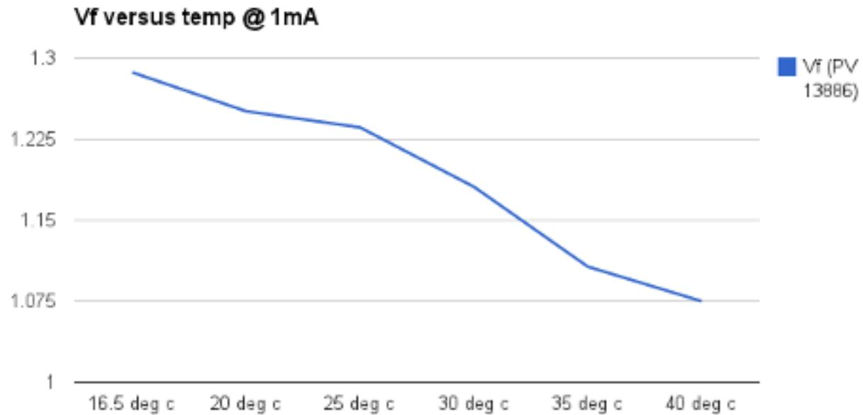
10v through 10K resistor. Temperature adjusted with air dryer and measured with laser temperature probe
