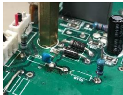
Shaping capacitor leg.
