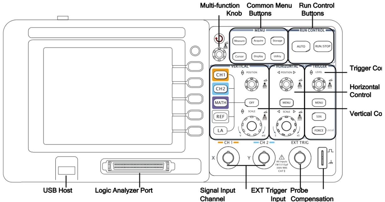
*Figure 1. Front Panel of the Oscilloscope*
