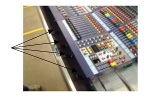
STEP 2 - Lift the module up and Remove the ribbon cables (ensure a note is made of were each cable plugs)
