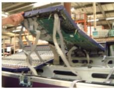
STEP 3 - Bring the module back almost vertical and them pull out in the direction of the arrow. (The rear of the module will fall from the mounting and can be pulled out about 15mm)
