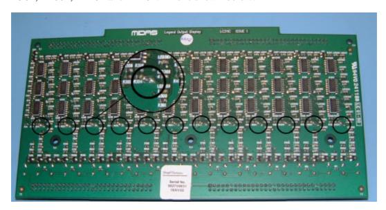
STEP 8 - Fit the capacitor between the left hands side of the resistor and the ground plain to the right of the resistors previously cleared of resist in the last step . The Capacitor we use is surface mount, part number CAP06-GK510050.
