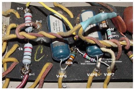
new 1M resistor directly from the V4b grid to ground, arching it up a bit so that it will not short against the eyelet. I have already unsoldered one end of the 0.1uF coupling cap connected to the cathode so that we can run a 2M2 bias resistor underneath it from the grid of V4b to B+3. I mention all of that because the layout of the 2M2 bias resistor and jumper is a bit
