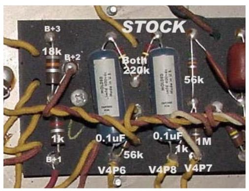
18k resistor in the power supply with a 4k7 resistor, which will raise the voltage to the PI even more. (He has many other mods that he would do to a PR like putting in a choke and replacing the 10" speaker with a 12" speaker.)
