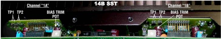
The 14B is comprised of four channels which are combined in pairs to form two bridged amplifier channels (Ch1 & Ch2). One such bridged channel is shown here. Because it is comprised of two channels (A & B) there are two pairs of test points and two BIAS trim pots, both of which must be set to the same levels. The same is repeated for the other bridged channel.
