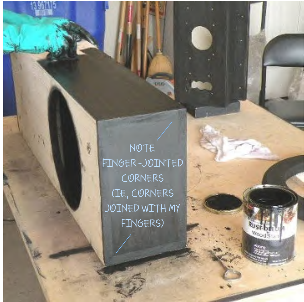
Impelling a Protective Coating into the Cellulose Components (STAINING THE CABINETS)
