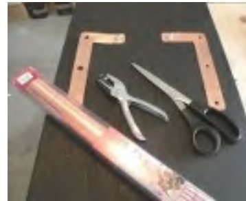
The Terminal Contacts (CUT, PUNCH, ATTACH)
