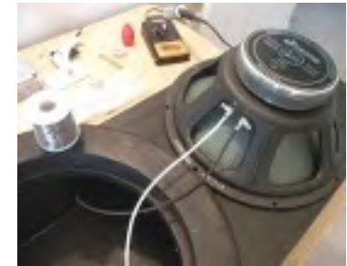
Transducer Connexions (SOLDER)
