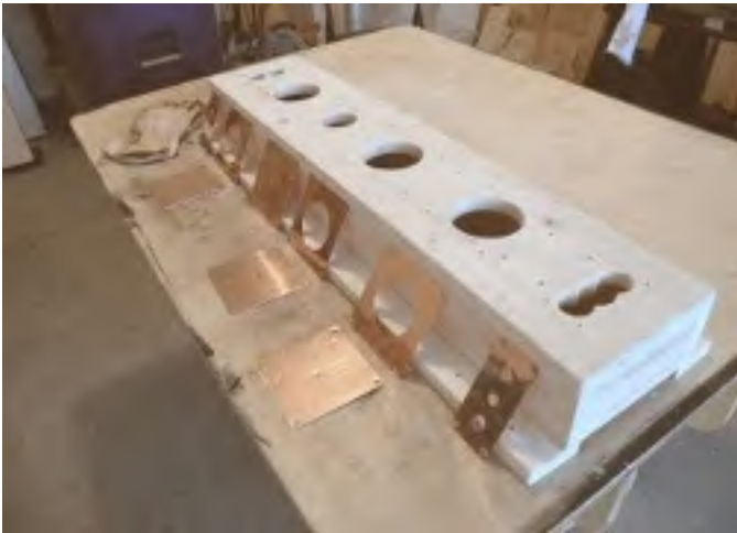
Bored Exposed Component Passageways (HOLES FOR JACKS, SWITCHES, TUBES, ETC)
