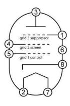
KT88 vacuum tube Beam Tetrode
