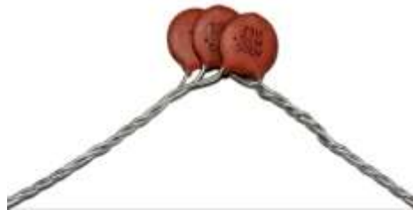
Figure 10b – Parallel .01 \mu F Capacitors
