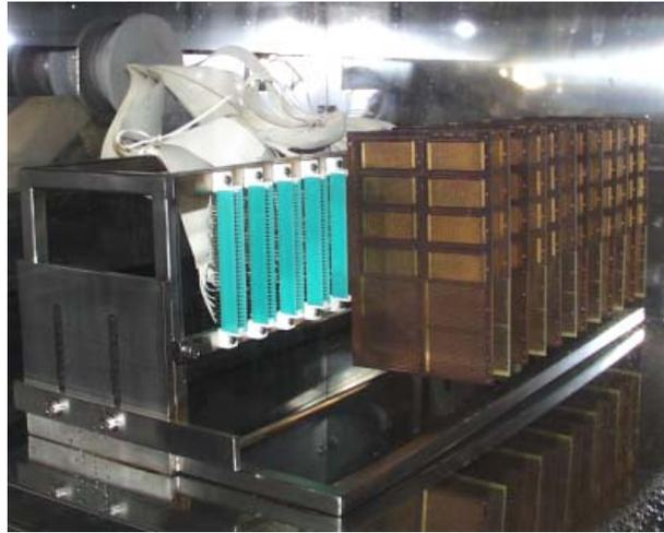
**Figure 12. CAF test coupons under test in environmental chamber.**
