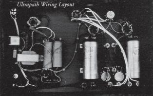
power supply capacitor, then through the cathode bypass capacitor to the tube. These capacitors are usually electrolytics and would be back to back or negative to negative. This seems strange now but it was the accepted, normal way to do it. Coupling back to the cathode with a capacitor from the end of the primary appeared to be practical, and was tried. Removing the cathode bypass capacitor seemed proper at this point.
