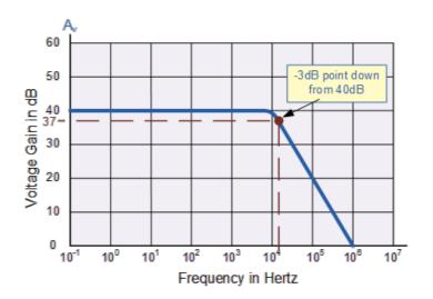
Here we have used the 40dB line as an example. The -3dB or 70.7% of Vmax down point from the frequency response curve is given as **37dB**. Taking a line across until it intersects with the main GBP curve gives us a frequency point just above the 10kHz line at about 12 to 15kHz. We can now calculate this more accurately as we already know the GBP of the amplifier, in this particular case 1MHz.
