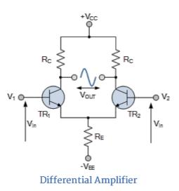
The circuit operates from a dual supply +Vcc and -Vee which ensures a constant supply. The voltage that appears at the output, Vout of the amplifier is the difference between the two input signals as the two base inputs are in *anti-phase* with each other.
