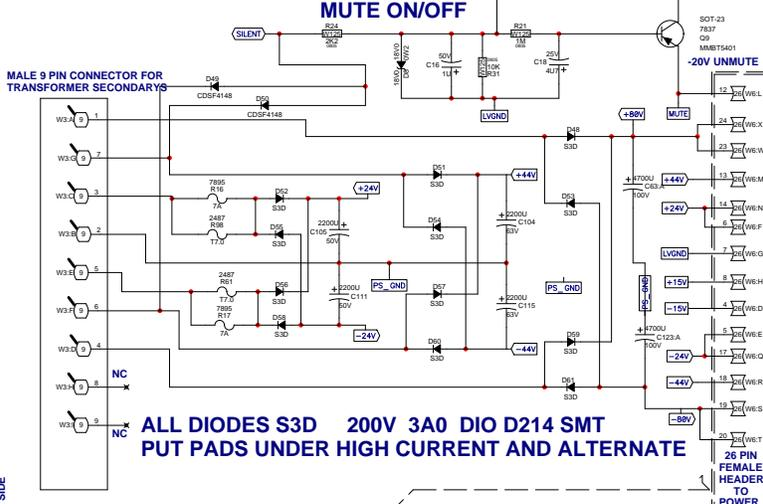
**ALL DIODES S3D 200V 3A0 DIO D214 SMT PUT PADS UNDER HIGH CURRENT AND ALTERNATE**
