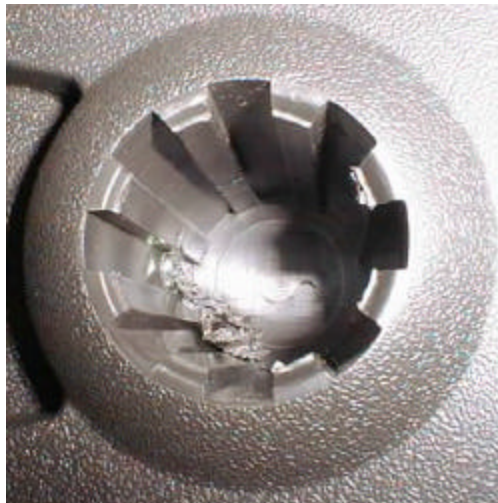
Plastic burrs from insert installation
