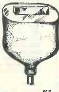
Fig. 3. The coil with protective rubber covering
