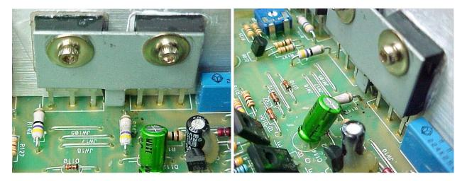
I have re-mounted and soldered in all the parts, but I still need to check all of the support devices due to this fault, and make sure I didn't also short anything else out. From these photos, it looks like I need to double-check that gate resistor, as it has overheated, enough that the black band has nearly disappeared.
