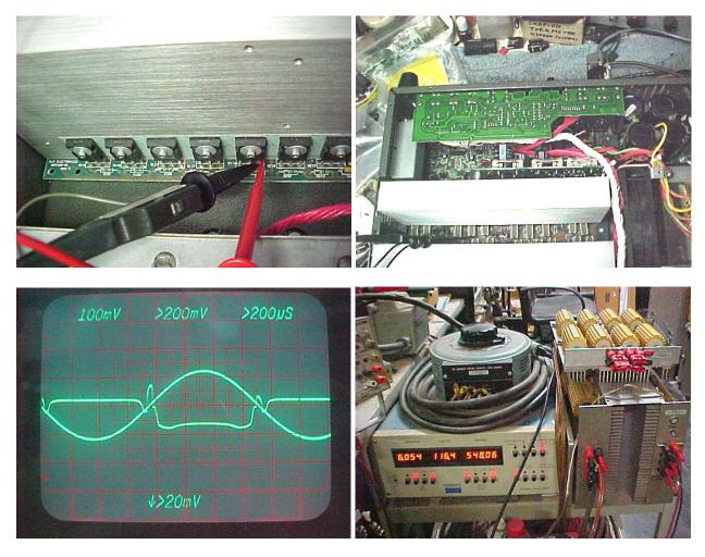
Getting at the back side of the amp channels requires removing the rear top PCB Assy
