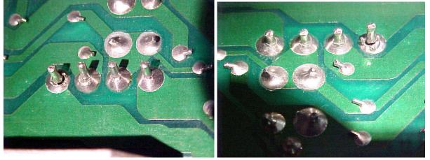
Desoldered, cleaned, resoldered bridge leads. Checked all Mosfets & drivers for blown devices, all ok. Also found two phone jacks on main PCB with solder fractures...repaired. Rest of PCB components ok, reassembled, powered up....130W @ 120VAC at idle. Amp working fine. Checked all functions, sounds nominal.
