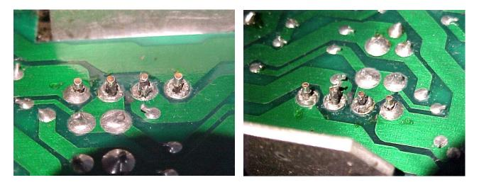
Removed power amp pcb assy, and again, close inspection of circuit board solder joints revealed same severe solder fractures on all 4 leads of main bridge rectifier
