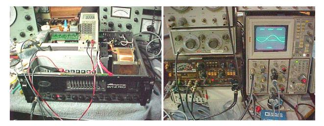
The waveshape seen differentially across the source resistor is NOT sinusoidal, but rather an offset squarewave, with artifacts.
