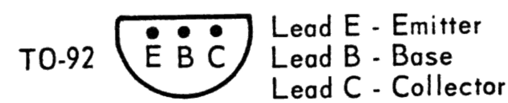
Figure 5. Typical Transistor Package Sizes
