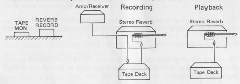
With TAPE MON pressed in and REVERB RECORD out the playback signal is reverb processed.
