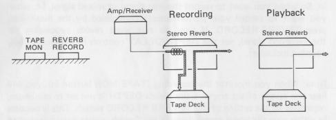
With both TAPE MON and REVERB RECORD pressed in, the record signal is reverb processed.
