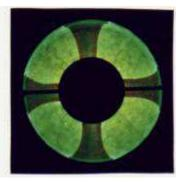
The luminous disk of 6E5 has a single line of shadow that passes 90 degrees, no signal received, a gradual closure giving a full circle on a strong station.
