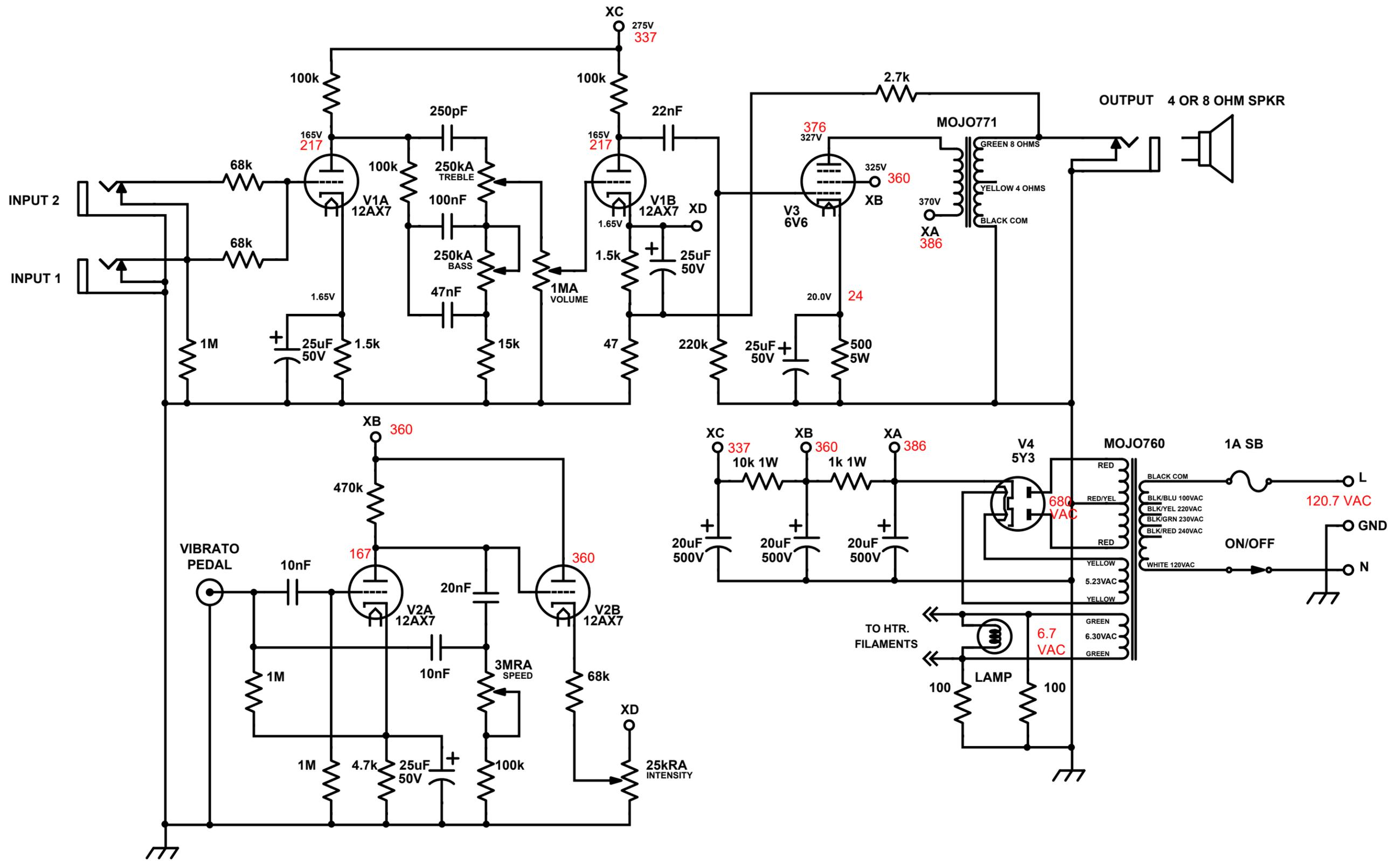
All resistors are rated for 1/2W unless specified.
