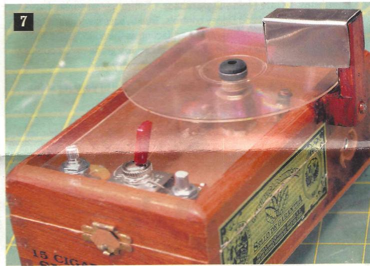
when designing the layout of the top. Mount the DC motor to the underside of the clear disc/lid; drill a 3-millimeter centered-access hole 2" from the top edge of the lid. Then, use a two-part epoxy that dries clear to secure the motor. Allow it to dry for an hour, making sure the motor body is perfectly parallel to the plane of the lid, so it won't wobble when rotating.
