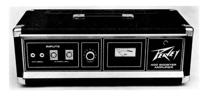
The new 400 Booster Power Amplifier uses eight high voltage 30 amp power devices to reliably deliver 200 watts RMS into 4 ohms with less than 0.1% THD from 20 Hz to 20 kHz. The 400 Booster can also deliver 310 watts RMS into a 2 ohm load just as reliably. The output devices are mounted on a massive aluminum heatsink for continuous duty. Additional thermal protection is afforded by our thermal conpen-
