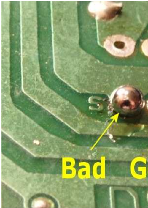
An example of a "dry" joint – the solder failed to flow, and instead beaded to form globs of solder around the wire.
