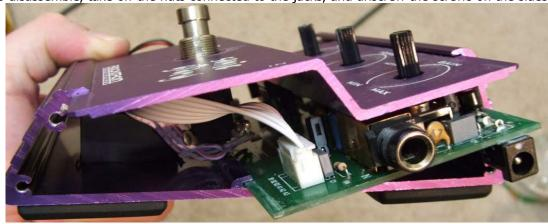
Also, make sure you unscrew the switch, take off the knobs, and slide the bottom out and away
