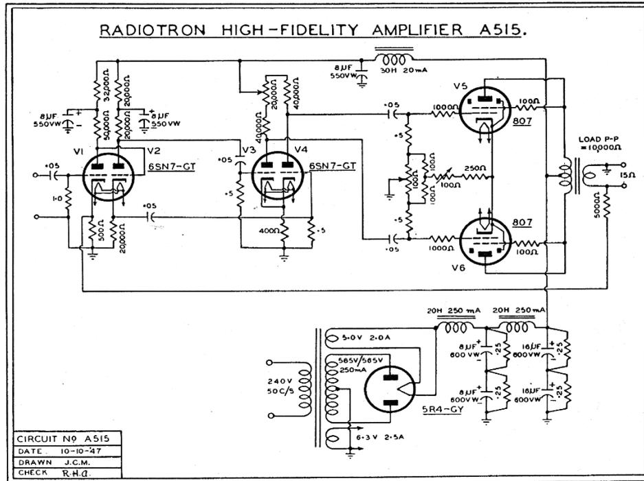
1947-8. The A515 circuit format of the *Williamson* amplifier as developed by the AWW Laboratory, Sydney, with double triode 6SN7 valves for input and type 807 valves for the output stage. It is functionally essentially identical to the original.
